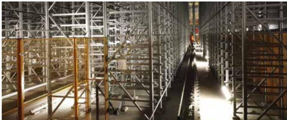
Because of the low oxygen nature of the freezer, all pallets in and out of the freezer are handled by an automation system comprised of conveyors, monorails and cranes. (Photo courtesy of Fisher Construction Group.)
